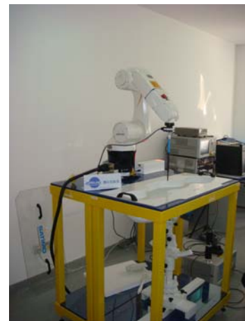
图 2: Open SAR 测试系统 Figure 2 (Open SAR&HAC test system)
